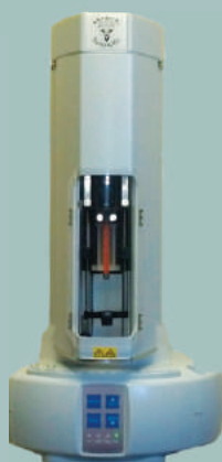
The HTA GC / HPLC Auto Sampler can inject into 1 or 2 injection ports sequentially. It also has 6 solvent and 1 waste positions
