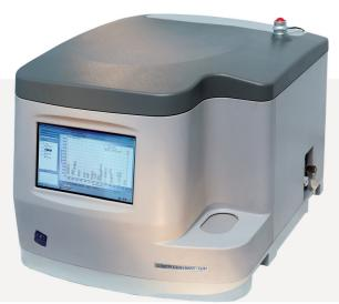
The principle of the spectrometer operation is as follows. A sample is irradiated by X-ray tube primary radiation, then the intensity of the secondary fluorescence from the sample at wavelengths corresponding to the elements to be detected is measured, and the subsequent calculation of the mass fraction of these elements is done. For the last operation, a pre-built calibration characteristic is used, which is the dependence of the element content from the measured intensity.
