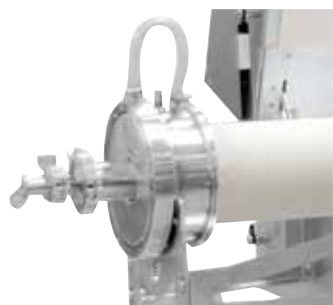
Water-cooled stainless steel flange
