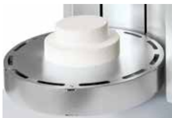
Electrically driven lift-bottom
