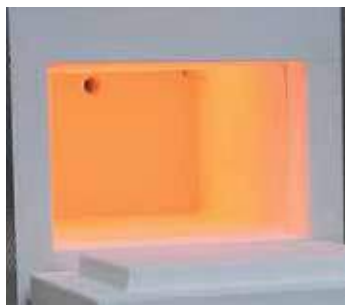
Muffle heated from four sides
