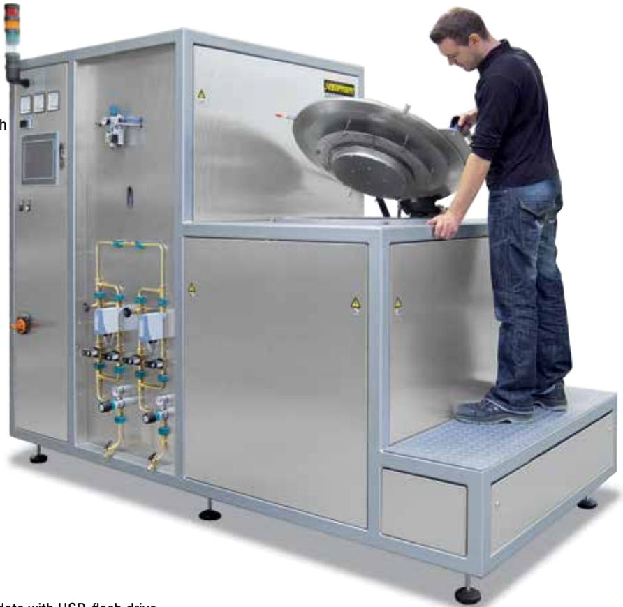
Retort furnace SVHT 9/24-W with tungsten heating
