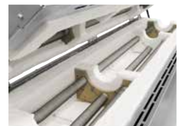
Tube furnace RSH 120/1000/11S, three-zone controlled, incl. zone separators to reach a temperature gradient
