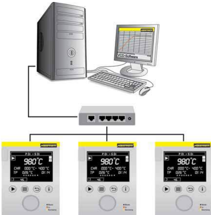
Example lay-out with 3 furnaces
