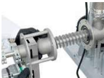
Screw-conveyor with adjustable speed
