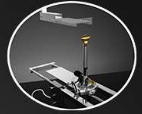
94 HBF, HF-1, HF-2: Horizontal Burning
